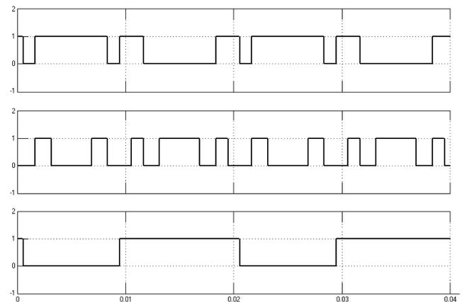
Figure 8 Cross Switch Inverter SHE-PWN Switching Pulses (S1, S3, S5)
