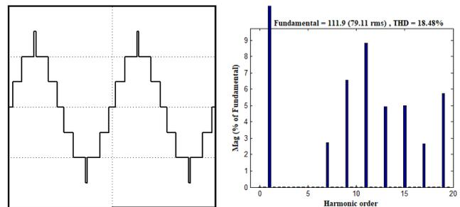
Figure 11 SHE-PWM a) output voltage, b) THD and fundamental, at  $m = 0.4$
