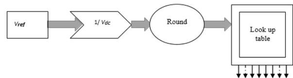
Figure 4 NLC Flow Diagram
