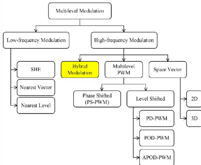
Figure 1 Classification of MLI Control Method
