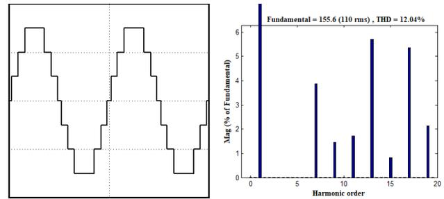
Figure 10 SHE-PWM a) output voltage, b) THD and fundamental, at  $m = 1$
