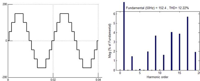
Figure 12 NLC a) output voltage, b) THD and fundamental, at  $m = 1$
