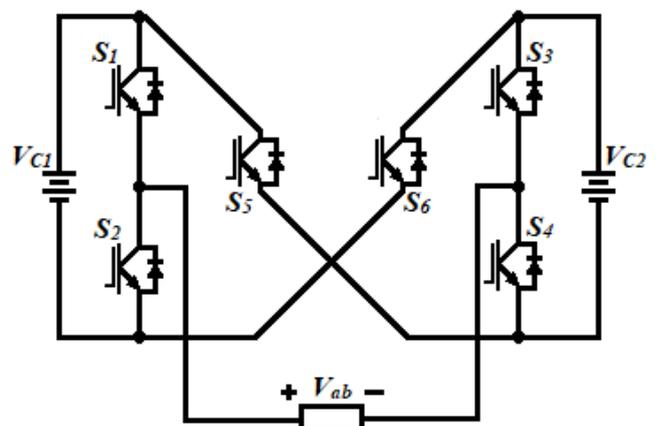
Figure 3 Cross Switch Inverters
