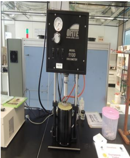
Fig 3.1 HPHT Viscometer used to measure Viscosity
