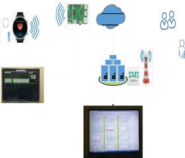
Figure. 3 system architecture for heart rate monitoring using IoT [2]
