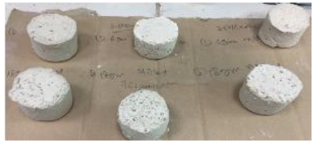
Fig. 3.3: Ceramic bodies after drying (Millet)
