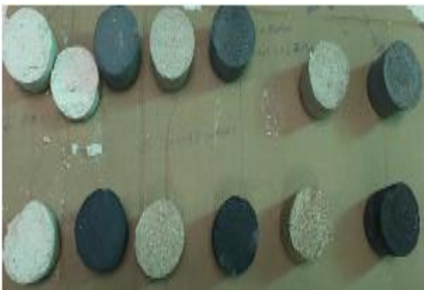
Fig. 3.2: Ceramic bodies after drying (Saw dust and Charcoal)
