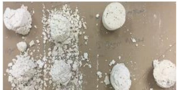
Fig. 3.5: Porous ceramic bodies with (Millet) after firing
