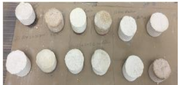
Fig. 3.6: Porous ceramic bodies with Saw dust and Charcoal after firing
