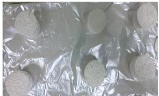
Fig. 3.7: Porous ceramic bodies with Poppy seeds after firing
