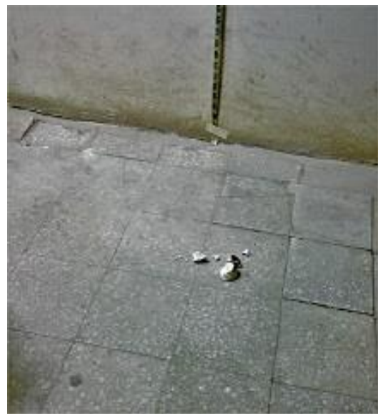
Fig. 3.11: Charcoal porous ceramic bodies drop test
