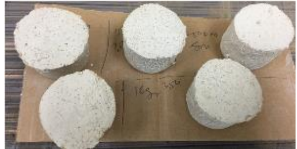
Fig. 3.4: Ceramic bodies after drying (Poppy seeds)
