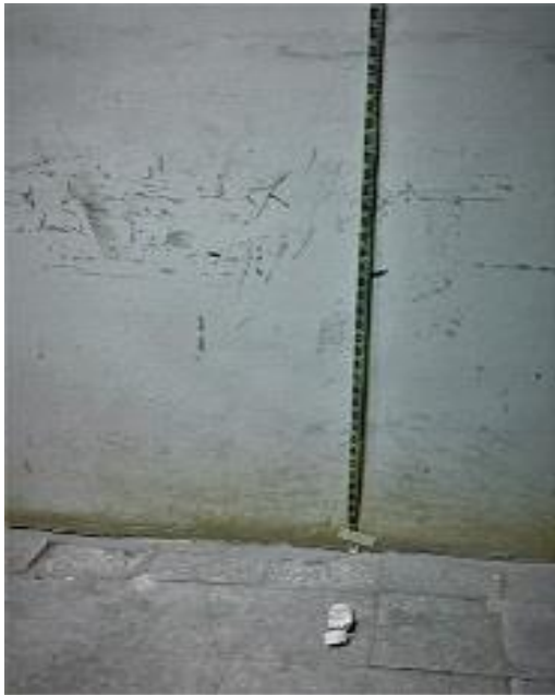
Fig. 3.8: Sawdust Porous ceramic body drop test
